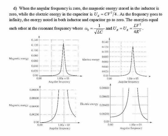
**31.50:** a) Since the voltage drop between any two points must always be equal, the parallel LRC circuit must have equal potential drops over the capacitor, inductor and resistor, so  $v_R = v_L = v_C = v$ . Also, the sum of currents entering any junction must equal the current leaving the junction. Therefore, the sum of the currents in the branches must equal the current through the source:  $i = i_R + i_L + i_C$ .
